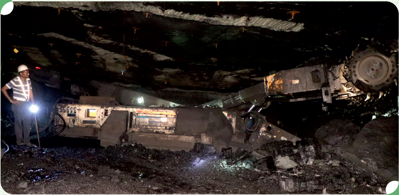
■ Continuous Miner in operation at one of Underground Mine, WCL.
