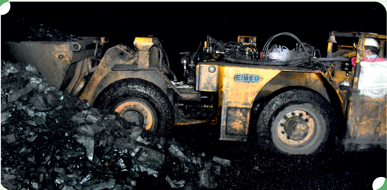
■ LHD Machine in Operation at Chhatarpur-I UG Mine, Pathakhera Area.
